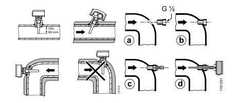
NOTICE! For sensors with non-sealing threaded nipples G  $\frac{1}{2}$ , use a sealant with the threaded connection (for example, hemp, Teflon tape and so on).
