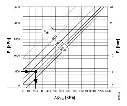
$\Delta p_{max}$  = Differential pressure at a nearly closed ball valve
