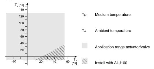
Only use GDB.., GDD..,GSD.. and GQD.. actuators at medium temperatures > 0 °C.
